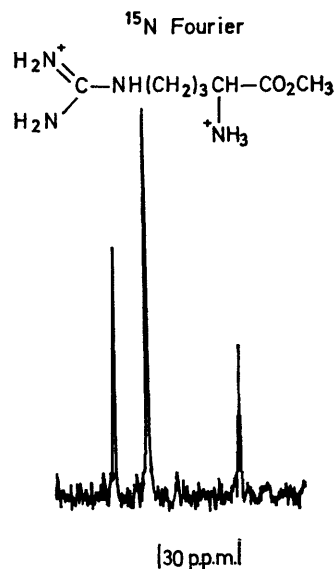
FIGURE. Natural abundance, proton-decoupled ^{15}\text{N} "Fourier" power spectrum of arginine methyl ester di-hydrochloride at 21.14 kg. The spectrum is the result of 66,680 pulses each of 6 \mu s duration and repeated every 0.4 s.
